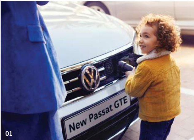
01 The large capacity 13 kWh battery increases the electric-only range up to 34 miles 2 of emission-free driving . Charging time is around four hours, while new driving modes allow you to save battery use for zero-emission zones. For drivers commuting into London, the new GTE is exempt from the Congestion Charge. Model shown is new Passat Estate GTE with optional premium signature paint.
